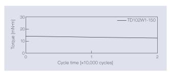
Measurement of torque at a rotation speed of 20 min<sup>-1</sup>
